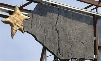
Reproduction of a block of slate made from composite material © CRITT material
