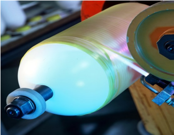
Manufacturing a part by filament winding. © EADS Composites Aquitaine
